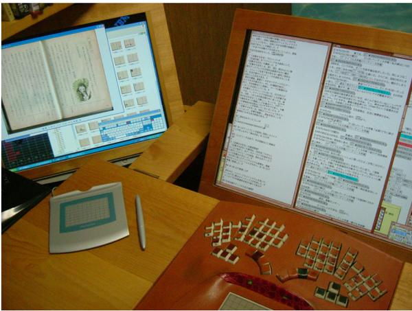
Figure 1. LCDs embedded into the library desk. The left display slide-shows digitized images.
