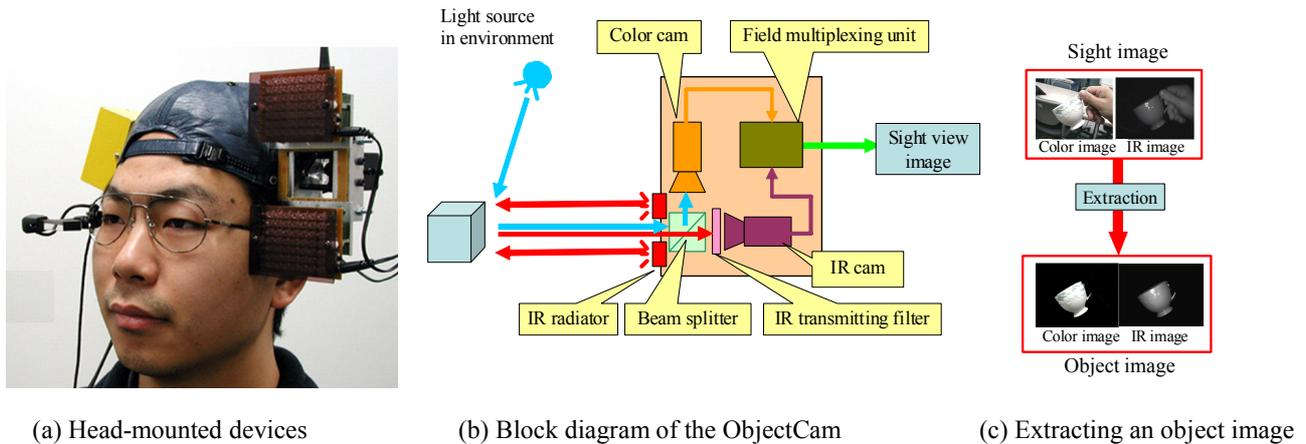
Figure 4: Overview and configuration of the ObjectCam
