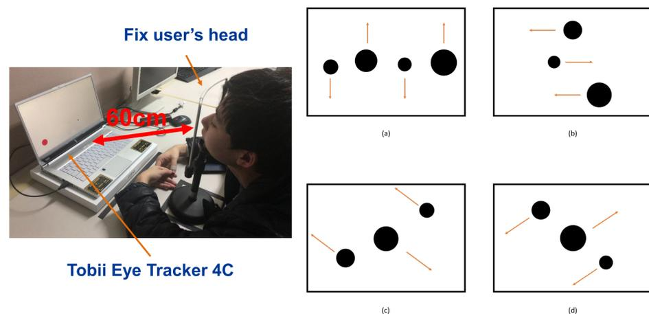
Figure1. Experiment setup (left) and four types of moving target which the participants require to acquire (right)
