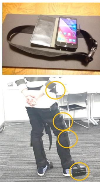
Figure 3 Measuring unit and its installation example
