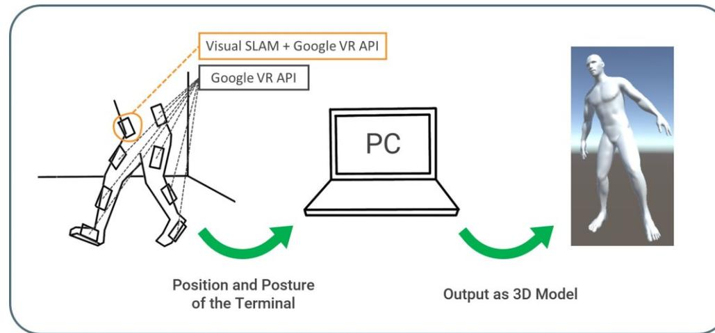
Figure 6 Schematic of demonstration system
