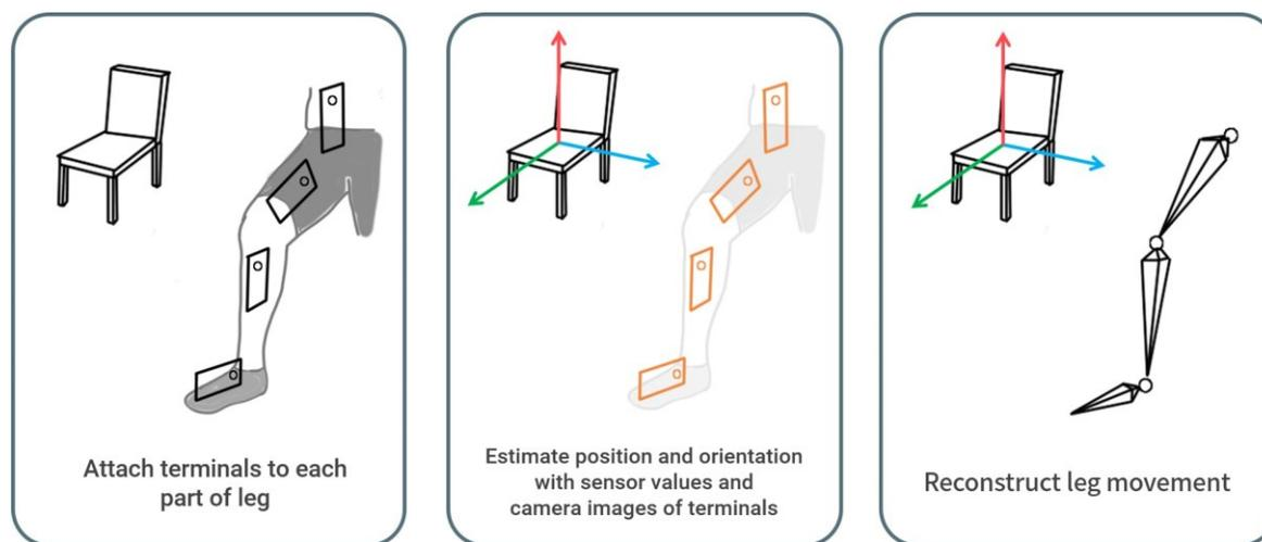
Figure 4 Schematic of measuring system
