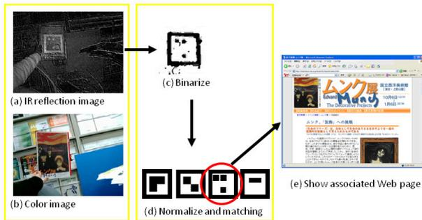
Figure 2: System Diagram
