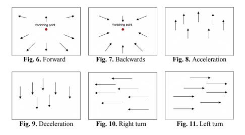
Details of optical flow pattern for each running state is described as follows.
