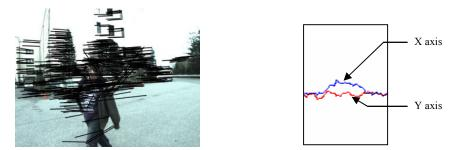
Fig. 17. Two sensors data when a moving object does not reflect (turning right)
