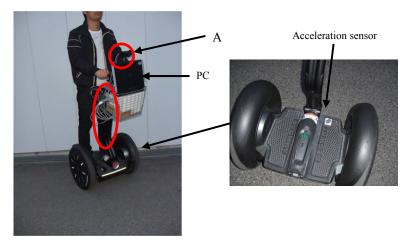
Fig. 2. Placement of sensors on the Segway
